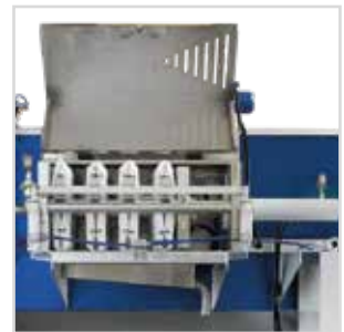
Hot-dip galvanized filter press with stainless steel cover and drain channel.
