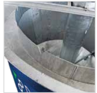
Overflow pipe for clarified water on the upper part of the cylinder.
