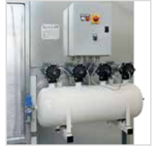
Compressed-air tank, needed for the cleaning system by counter-blowing.
