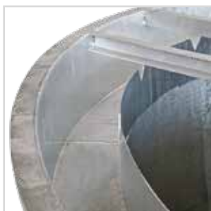
Overflow pipe for clarified water on the upper part of the cylinder.
