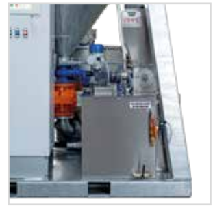
Station for the preparation and automatic dosing of the flocculant solution.
