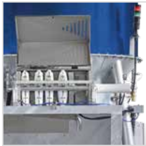
Hot-dip galvanized filter press with stainless steel cover and drain channel.
