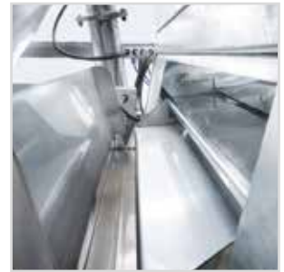
Water collection system from filter press with automatic dripping tray.
