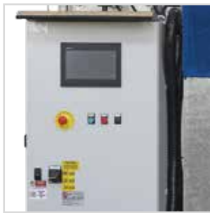
Control panel with 10" touch screen managing all the plant operations.
